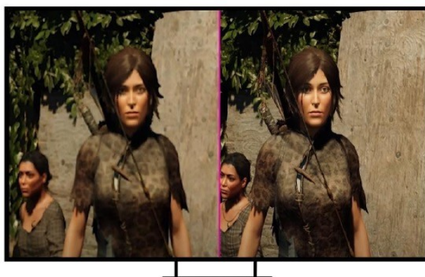
Figure 3 Example of degradation of image quality when streaming due to packet loss (the left one) on the case of the game Shadow of the Tomb Raider
