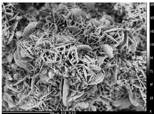
Obr. 4 – Krystaly sádrovce na povrchu pískovce. Cameca SX 100. Foto P. Sulovský. Fig. 4 – Gypsum crystals surface on the sandstone. Cameca SX 100. Photo P. Sulovský.
