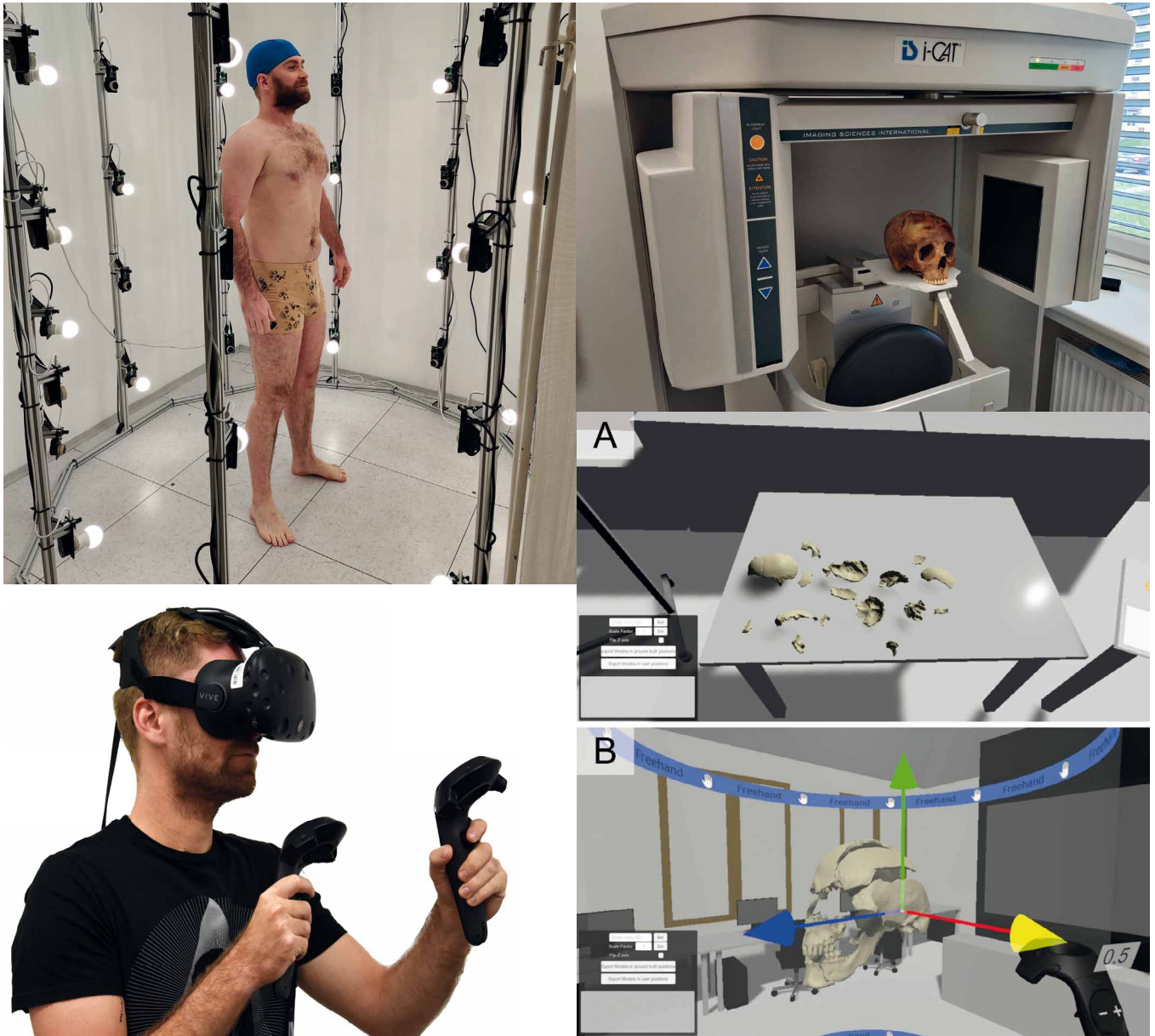
Fig. 4. Multi-camera photogrammetry system (top left), a human skull examined using a CT unit (top right), virtual reality workspace for assembling fragmented skeletal remains (bottom).
