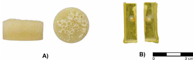
Figure 4: A) Strong exothermic reaction between dental sample and its embedding medium (Duracryl Plus). Tooth embedded in a similar block lacks visibility and the sample is thus destroyed. B) Yellow coloration occurs in the embedding medium (Dentacryl) after its solidification. Colour change in such a degree is inappropriate due to the low visibility of cut line in dental samples and misinterprets observed taphonomic phenomena.
