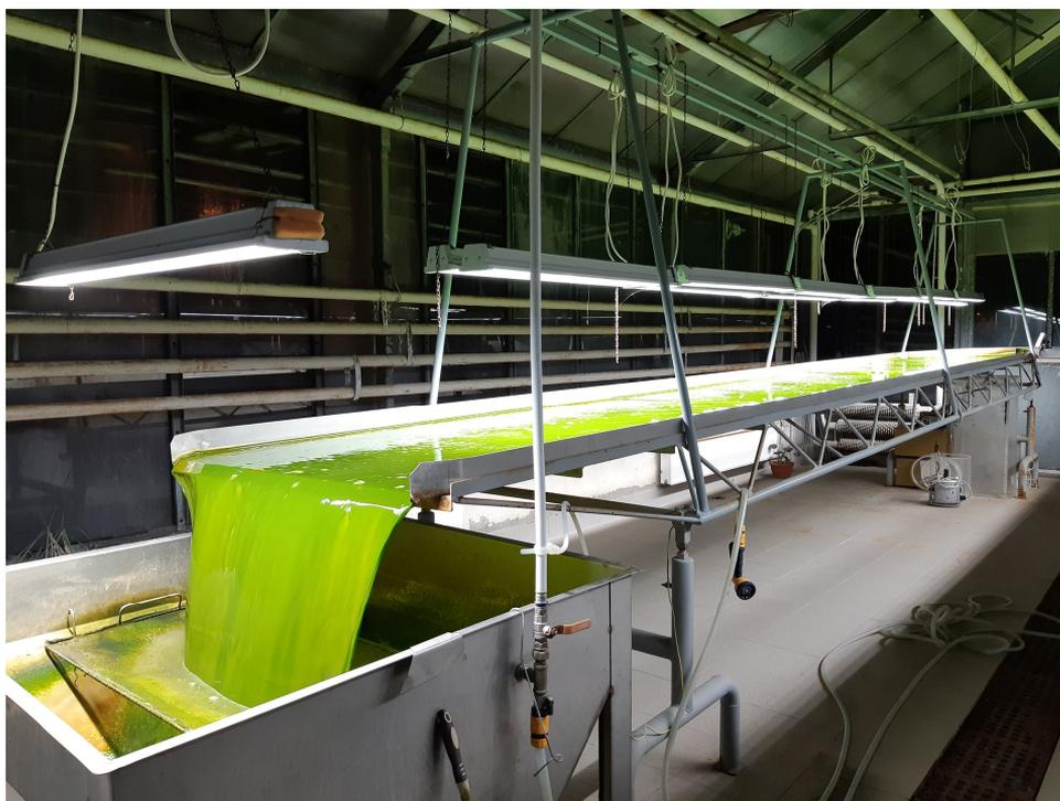
**Fig. 1.** The night LED illumination of the large-volume (150 L) thin-layer photobioreactor at the Institute of Botany CAS, Třeboň, Czech Republic.
