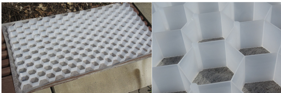
Fig. 3. BERA Gravel Fix™ – a reference gravel stabilization sheet; non-exposed.
