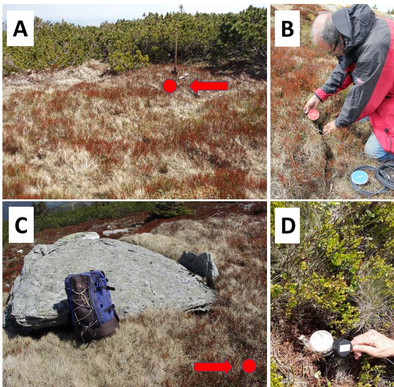
**Fig. 1.** The sites at which the heat flux sensors were installed in May 2020 in the Jeseníky Mts., 1 445 m a.s.l. The sites are indicated by a red dot. A – the spot located close to a *Pinus mugo* stand (abbreviated as PMUGO in the text), B – insertion of the sensor plate into a soil profile, C – the spot denoted as OPEN in the text, D – downloading data from a datalogger by an IR port.
