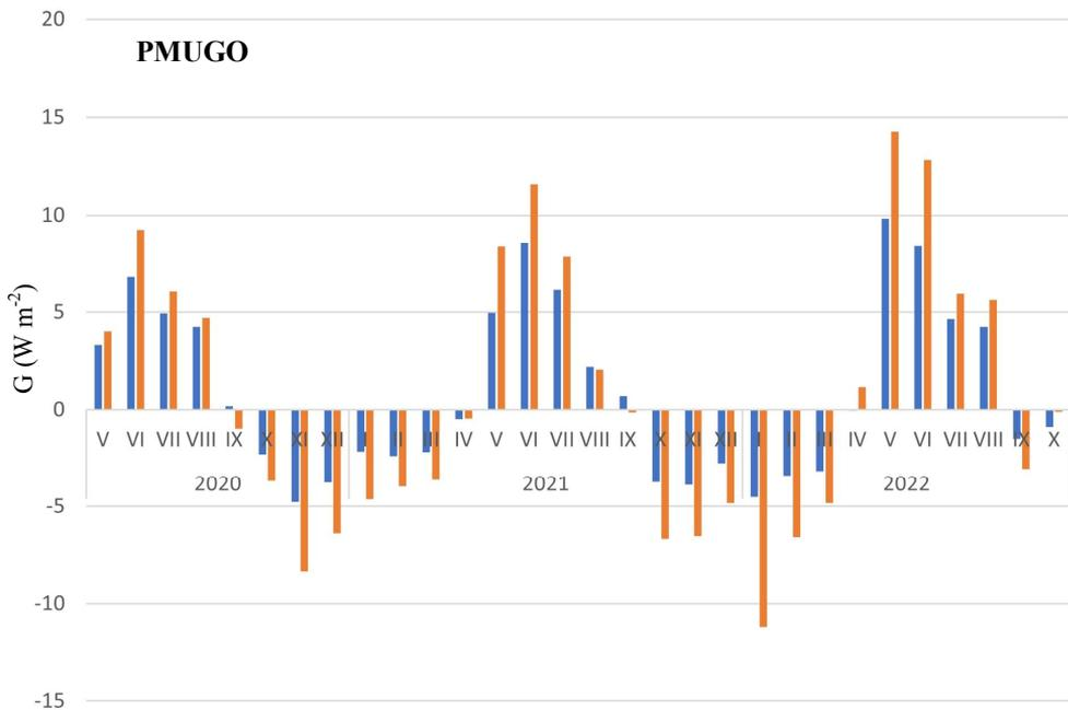
**Fig. 6.** Monthly means of soil heat flux ( $G$ ) for the PMUGO plot with grass vegetation with neighbouring dwarf pine (*P. mugo*), the Tabulové skály Rocks (1 445 m a.s.l., Jeseníky Mts.).  $G$  was measured by the sensors buried in the depth of 5 cm (orange columns) and 10 cm (blue columns).
