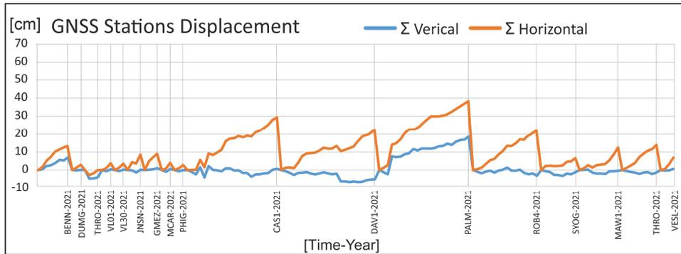
**Fig. 4.** Horizontal and vertical displacement graphic of GNSS stations in Antarctica continent.
