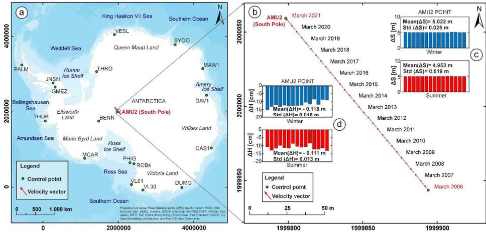
**Fig. 1.** a) Location of control stations (UPS-South), b) velocity vectors, c) distance and d) height differences of South Pole, AMU2 station (2006-2021 winter-summer).
