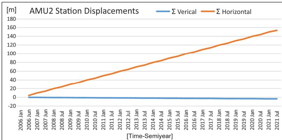
**Fig. 3.** Horizontal and vertical displacement graphic of AMU2 (South Pole) station (2006–2021).
