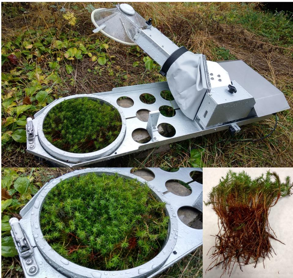
**Fig. 1.** Automated Soil CO<sub>2</sub> Exchange System (ACE) with the samples of *Polytrichum commune* installed in exposition collar.
