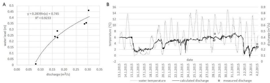
**Fig. 5.** Discharge from Phormidium Lake **A)** rating curve for Phormidium Lake outlet; **B)** discharge and water temperature time series together with manually measured discharge.
