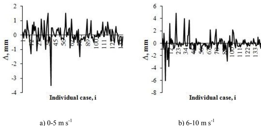
**Fig. 1.** Differences between records of Tretyakov gauge and Geonor T200-B gauge for solid precipitation during period of parallel measurements under different wind speed conditions. ( $\Delta = \text{Tretyakov g.} - \text{Geonor T200-B}$ )
