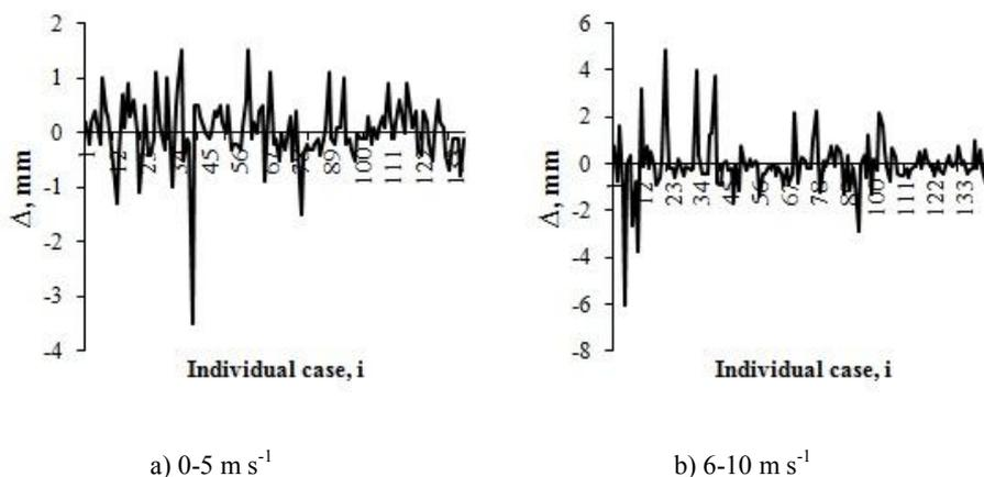
**Fig. 1.** Differences between records of Tretyakov gauge and Geonor T200-B gauge for solid precipitation during period of parallel measurements under different wind speed conditions. ( $\Delta = \text{Tretyakov g.} - \text{Geonor T200-B}$ )
