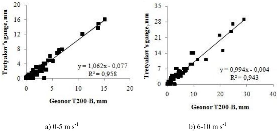
**Fig. 2.** Linear regression analysis for Tretyakov gauge adjustment to GEONOR T200-B for different wind speed ranges.
