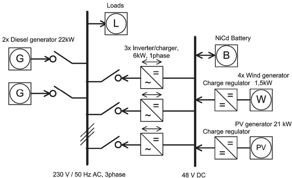
**Fig. 3.** Scheme of the new modified energy supplying system of J. G. Mendel station.
