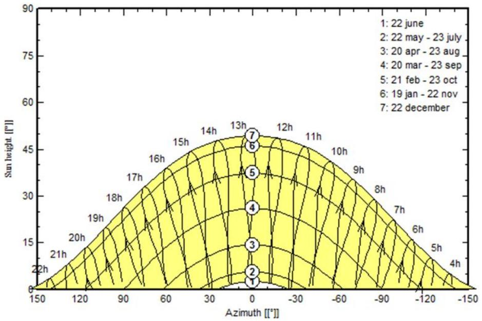
Fig. 4. Sun elevation angles, the paths for the J. G. Mendel station (created by PVsyst software).
