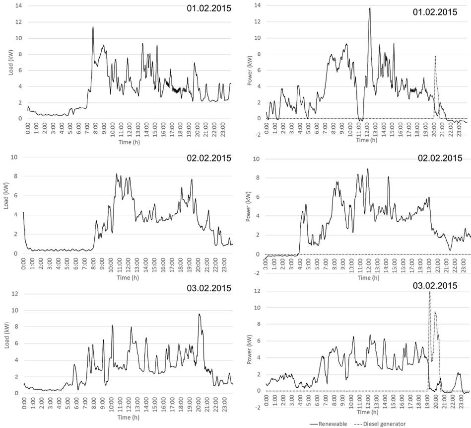
**Fig. 6.** Daily profiles of the electrical energy load (left) and generation (right).
