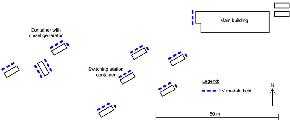
**Fig. 2.** Layout of J. G. Mendel station and location of PV system.
