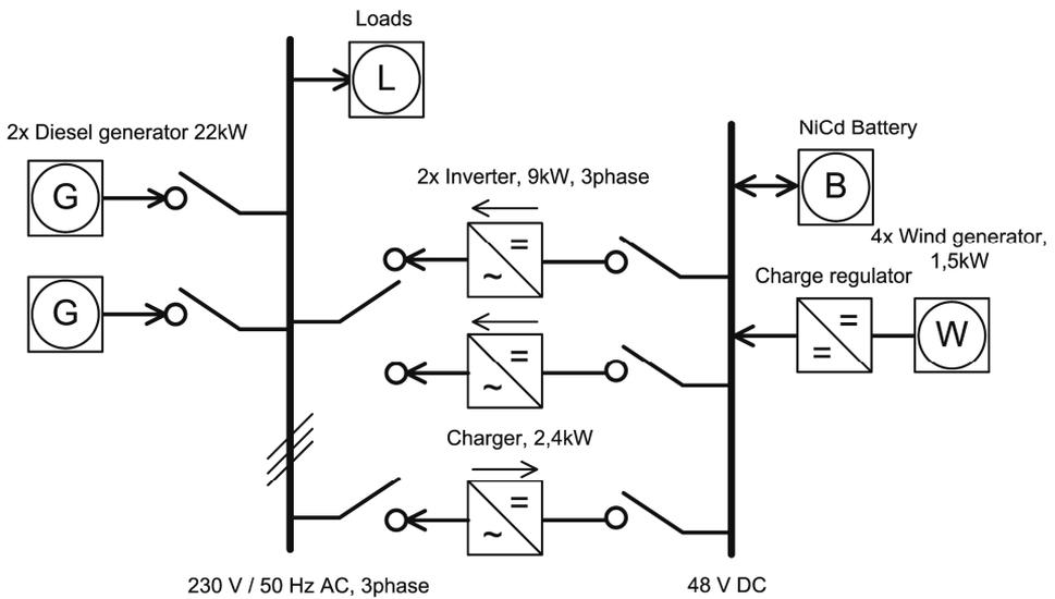
**Fig. 1.** Scheme of the original energy supplying system of J. G. Mendel station.
