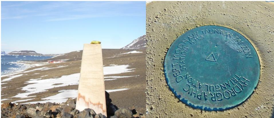
**Fig. 3.** Example of British stabilised points (Nr. 4001).
