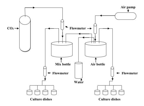
Fig. 3. The technical set up of the experiment. An apparatus shows a system for maintaining constantly elevated  $CO_2$  concentration.
