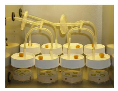
Fig. 1. Cultivation dishes with algal cells on glass microfiber filters. Three filters were placed in each of dishes.
