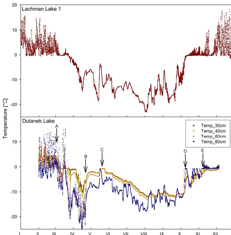
**Fig. 2.** Yearly courses of water temperature recorded in Lachman Lake 1 at the depth of 0.3 m (above), and Lake Dulanek (below) at different depths. The sensors were installed 30, 40, 60, and 80 cm above bottom. The uppermost one (Temp\_80) remained above water level for the whole year 2011. The lowest two (Temp\_30, and Temp\_40) remained within water columns for the whole year. A, B, C, D, E denote important events - *see Results*.
